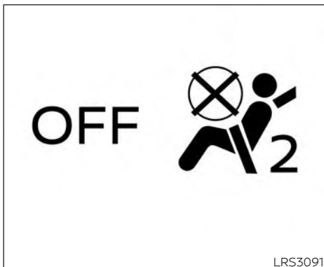
Front passenger air bag and status light
