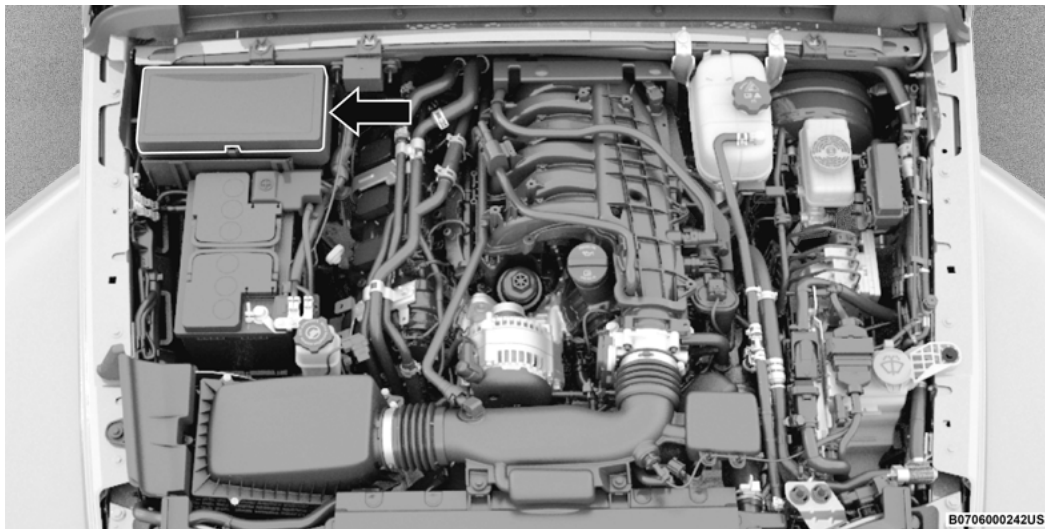
Power Distribution Center Location – Gas Engine
