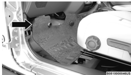
Front Carpet Pulled Away
