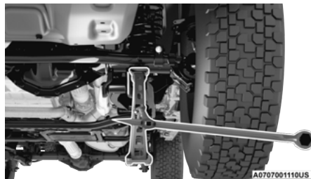
Front Jacking Location
