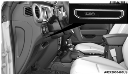
Power Inverter Switch (If Equipped)
