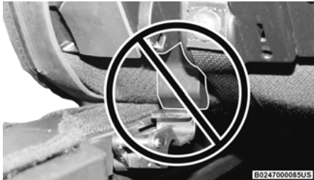
Incorrectly Seated Retainer
