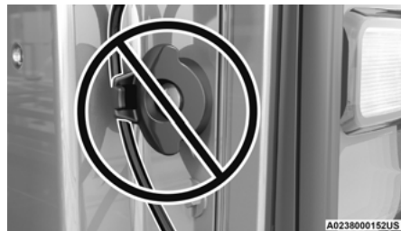
Incorrectly Seated Tailgate Strap
