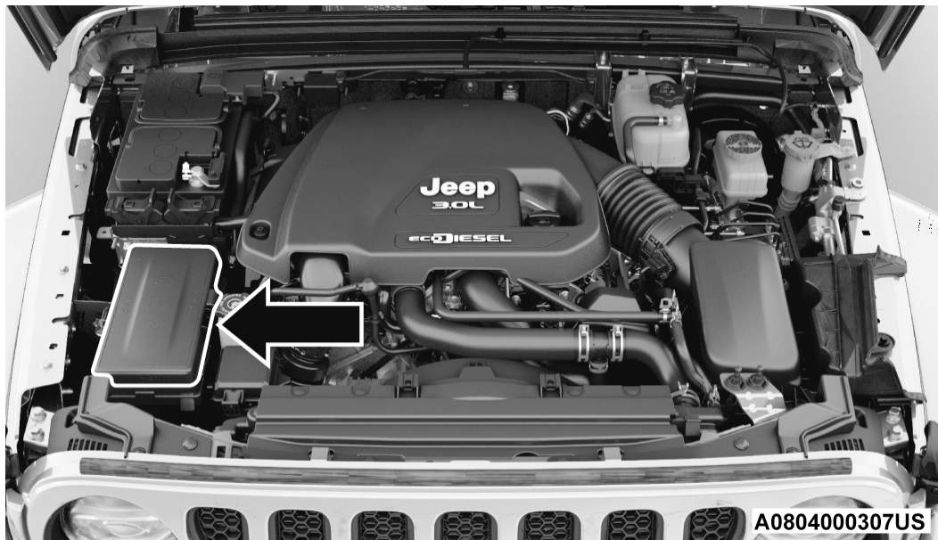
Power Distribution Center Location – Diesel Engine
