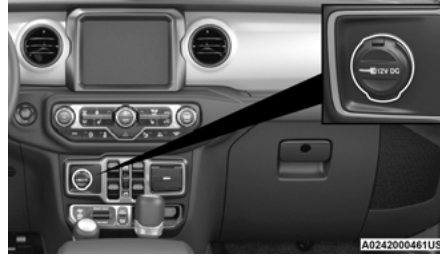
Front Power Outlet
