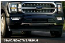
A Drag Reduction System (DRS) that actively streamlines the airflow under the truck to help improve aerodynamics.
