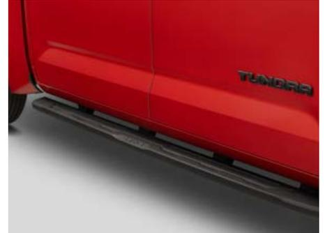
TRD cast-aluminum running boards
