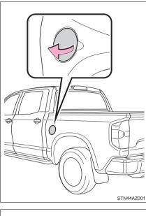
2 Turn the fuel tank cap slowly open, and hang the fuel tank cap on the back of the fuel filler door.
