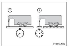
The gross trailer weight and kingpin weight can be measured with platform scales found at a highway weighing station, building supply company, trucking company, junk yard, etc.
