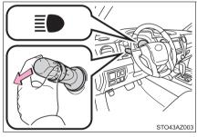
2 Press the Automatic High Beam switch.
