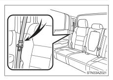
2 Pull and release the lever to unlock while raising the bottom cushion until it locks.
