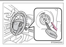
The steering wheel can be adjusted when (power adjustable type) The engine switch is in the "ON" position.
