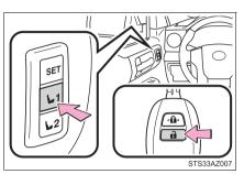
To prevent unintended triggering of the alarm, open and close a door once after a driving position has been recorded. (If a door is not opened within 60 seconds after is pressed, the doors will be locked again and the alarm will automatically be set.)
