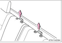
4 Route the top tether strap through the anchor strap router as shown in the illustration.
