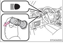
2 Press the Automatic High Beam switch.
