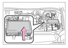
Under the instrument panel Remove the cover.
