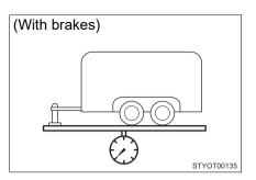
Additional optional equipment, passengers and cargo in the vehicle will reduce the trailer weight rating so as not to exceed GCWR, GVWR and GAWR.
