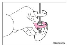
2 Using the wrench, tighten the antenna an additional 1/8th turn (20 to 45 degrees) to secure it in place.
