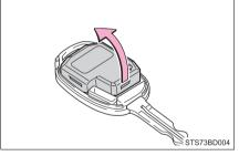
Open the case cover using a coin protected with tape, etc., and remove the depleted battery.
