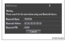
4 Register the Bluetooth<sup>®</sup> device using your Bluetooth<sup>®</sup> device.
