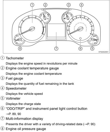
Displays the engine oil pressure
