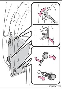
2 Open the fender liner and unplug the connector while depressing the lock release.
