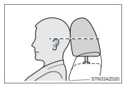
Adjusting the front center seat (bench type seat) and rear center seat head restraints (Double Cab and CrewMax models)
