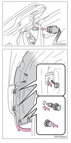
4 Reinstall the fender liner and install the screws and clips.
