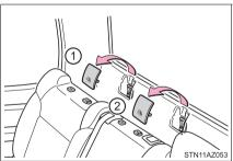
4 Latch the hook onto the anchor bracket and tighten the top tether strap.
