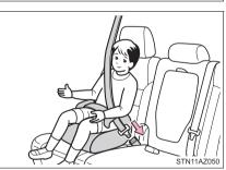
Check that the shoulder belt is correctly positioned over the child's shoulder and that the lap belt is as low as possible. ( $\rightarrow$ P. 32)
