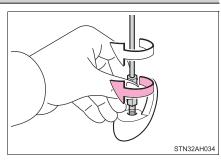
2 Using the wrench, tighten the antenna an additional 1/8th turn (20 to 45 degrees) to secure it in place.
