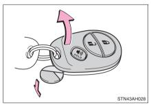
2 Remove the depleted battery.
