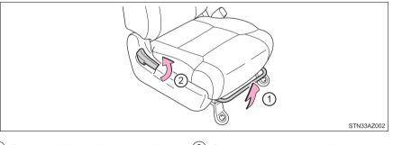
(1) Seat position adjustment lever 2 Seatback angle adjustment lever
