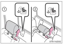
3 Remove the anchor bracket cover.
