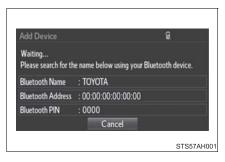
4 Register the Bluetooth<sup>®</sup> device using your Bluetooth<sup>®</sup> device.
