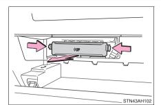
6 Pull the filter out of the filter outlet.
