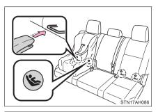
Seat belts equipped with a child restraint locking mechanism (ALR/ELR belts except driver's seat belt) ( $\rightarrow$ P. 34)
