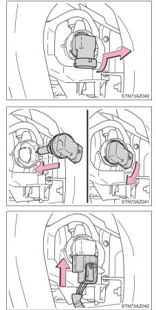
with the mounting, and insert. Turn it clockwise to set.
