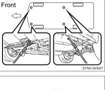
If you use chains or cables to tie down your vehicle, the angles shaded in black must be  $45^{\circ}$ .
