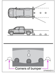
• Items which are located higher than the camera may not be displayed on the monitor.
