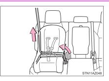
5 If the child restraint has a top tether strap, the top tether strap should be latched onto the top tether strap anchor.
