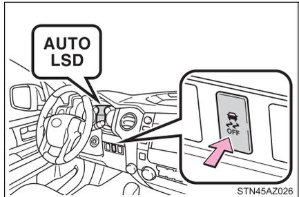
Stop the vehicle completely, and press the VSC off switch for more than 3 seconds.
