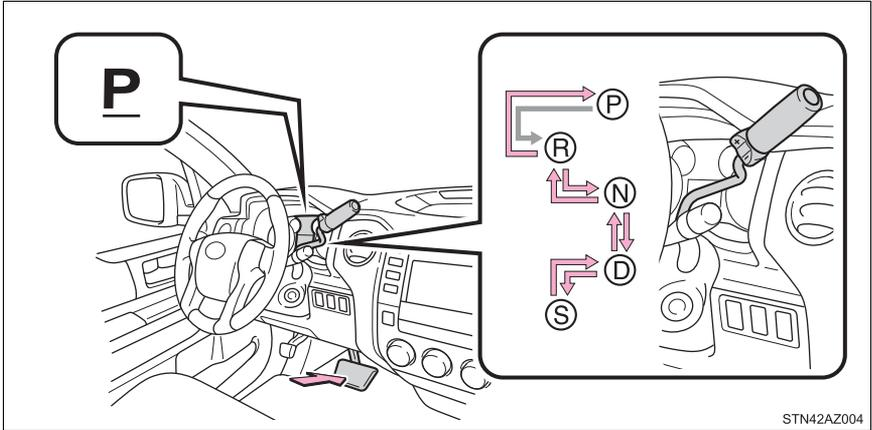
← While the engine switch is in the “ON” position, move the shift lever with the brake pedal depressed.
