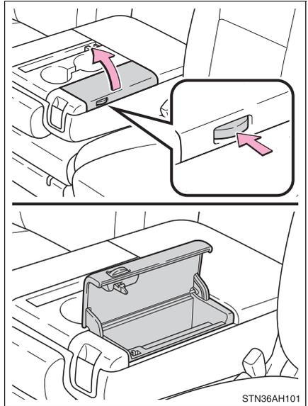
**Storage box (if equipped)****■ Using the storage box**
