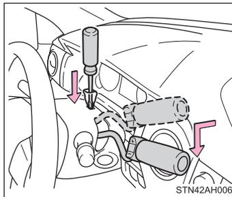
**■ If the “S” indicator does not come on even after shifting the shift lever to S**
