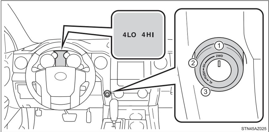
① "2WD" (high speed position, two-wheel drive)
