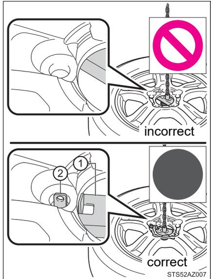
**3** Confirm it is not loose after tightening:
