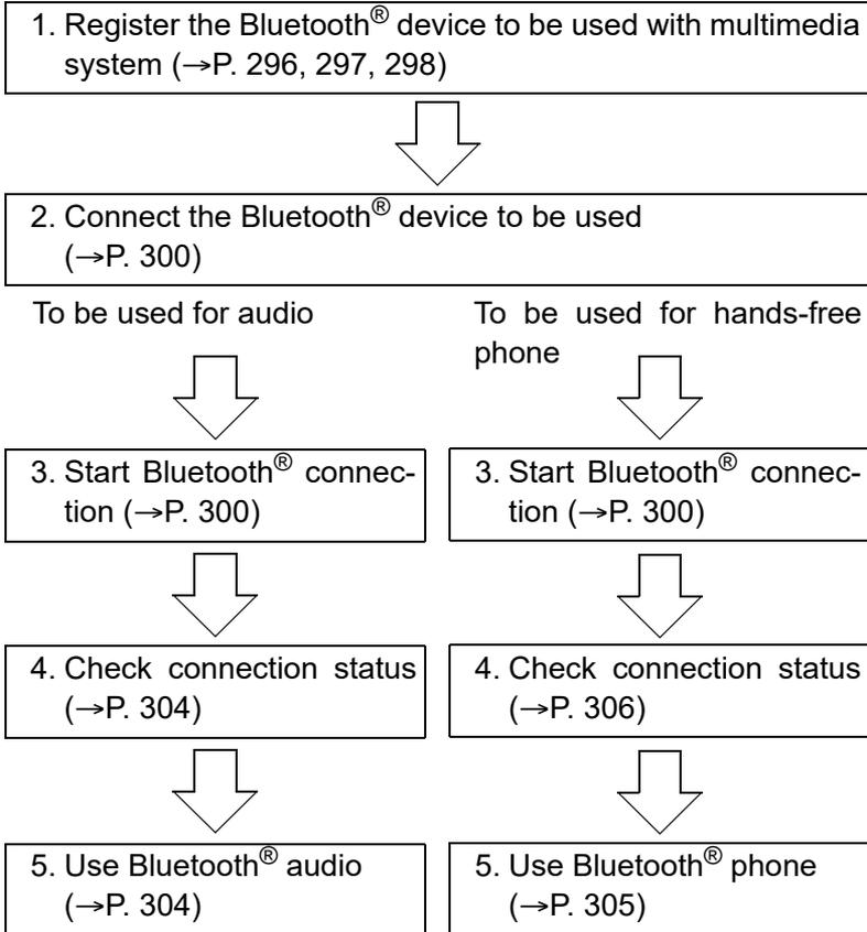
**Registering and connecting from the “Bluetooth Setup” screen**
