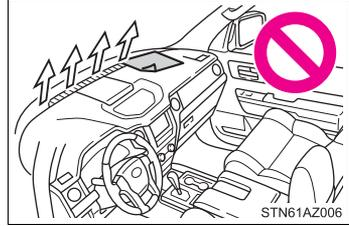
■ **To prevent burns (vehicles with rear view mirror defoggers and windshield wiper de-icer)**
