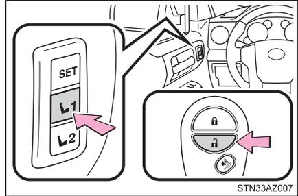
To prevent unintended triggering of the alarm, open and close a door once after a driving position has been recorded. (If a door is not opened within 60 seconds after
