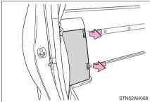
3 Unhook the rubber band and remove the tool bag.
