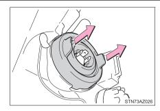
Release the bulb retaining spring.
