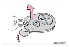
2 Remove the depleted battery. Insert a new battery with the "+" terminal facing up.
