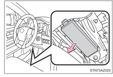
Remove the fuse with the pullout tool.
