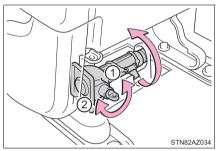
3 Unhook the rubber band and remove the tool bag.
