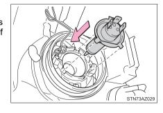
7 Install the bulb retaining spring.
