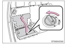
3 On vehicles with storage box, remove the jack cover panel.
