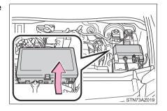
Under the instrument panel Remove the cover.
