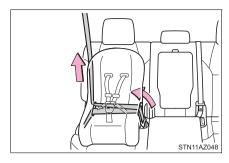
5 If the child restraint has a top tether strap, the top tether strap should be latched onto the top tether strap anchor. (→P. 68, 69, 72)
