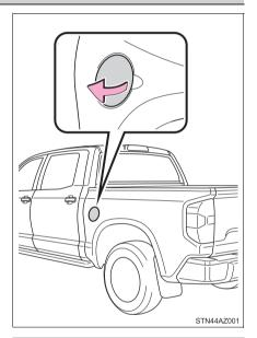
2 Turn the fuel tank cap slowly open, and hang the fuel tank cap on the back of the fuel filler door.
