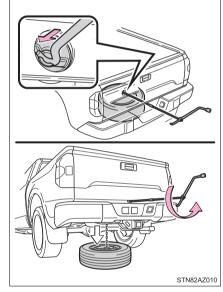
After the tire is lowered completely to the ground, remove the holding bracket.
