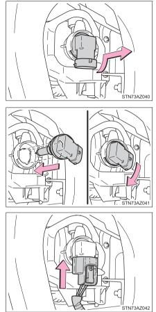
Align the 3 tabs on the light bulb with the mounting, and insert.
