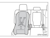
2 Run the seat belt through the child restraint system and insert the plate into the buckle. Make sure that the belt is not twisted.
