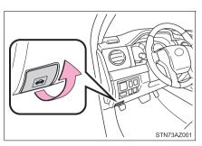
2 Pull up the auxiliary catch lever and lift the hood.
