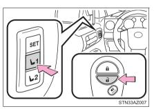
To prevent unintended triggering of the alarm, open and close a door once after a driving position has been recorded. (If a door is not opened within 60 seconds after recorded, the doors will be locked again and the alarm will automatically be set.)
