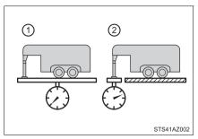
The gross trailer weight and kingpin weight can be measured with platform scales found at a highway weighing station, building supply company, trucking company, junk yard, etc.
