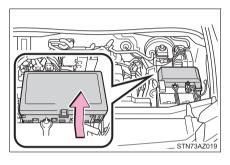
Under the instrument panel Remove the cover.
