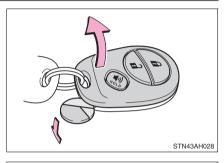
2 Remove the depleted battery.
