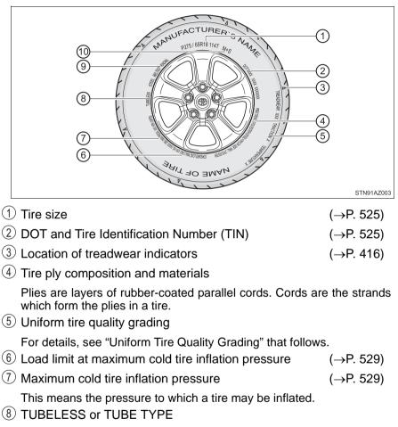
A tubeless tire does not have a tube and air is directly put into the tire. A tube type tire has a tube inside the tire and the tube maintains the air pressure.
