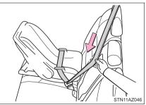
4 While pushing the child restraint system down into the rear seat, allow the shoulder belt to retract until the child restraint system is securely in place.
