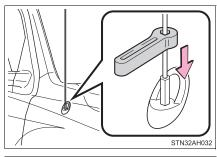
2 Loosen the antenna with the wrench and remove it.
