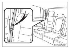
2 Pull and release the lever to unlock while raising the bottom cushion until it locks.
