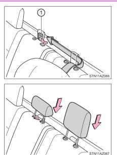
Child restraint systems with a top tether strap (CrewMax models)
