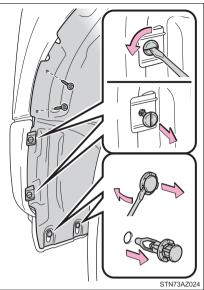
2 Open the fender liner and turn the bulb base counterclockwise.
