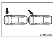
The SRS side airbags do not generally inflate if the vehicle is involved in a frontal or rear collision, if it rolls over, or if it is involved in a low-speed side collision.
