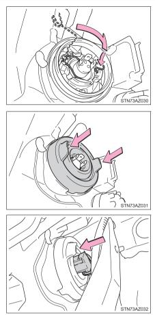
8 Install the rubber cover. When installing the rubb
