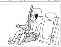
Check that the shoulder belt is correctly positioned over the child's shoulder and that the lap belt is as low as possible. ( $\rightarrow$ P. 32)
