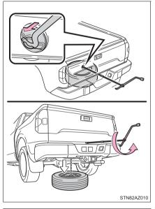
3 After the tire is lowered completely to the ground, remove the holding bracket.
