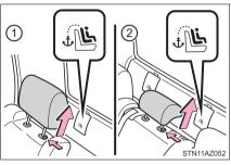
3 Remove the anchor bracket cover.
