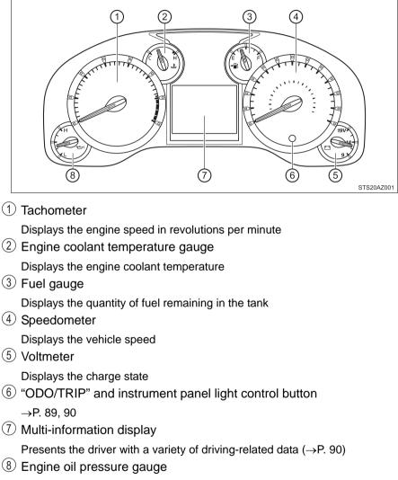
Displays the engine oil pressure
