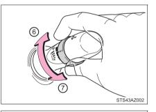
(8) Washer/wiper dual operation Wipers will automatically operate a couple of times after the washer squirts.
