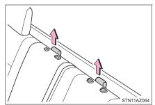
Route the top tether strap through the anchor strap router as shown in the illustration.
