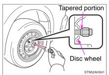
Replacing an aluminum wheel with a steel wheel
