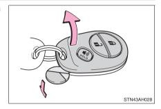
2 Remove the depleted battery.
