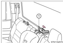
4 Latch the hook onto the anchor strap belt and tighten the top tether strap.
