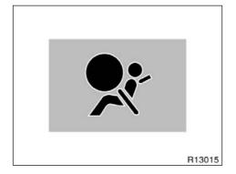
This indicator comes on when the ignition key is turned to the "ON" position. It goes off after about 6 seconds. This means the SRS airbags are operating properly.
