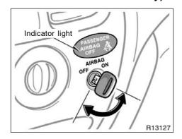
This on-off switch is designed to disable the passenger airbag in order to allow usage, if necessary, of a member of a passenger risk group identified in TABLE 1 is occupying the right front passenger seating position. (For details, see "SRS driver airbag and front passenger airbag" in this Section.)
