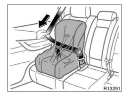
Fully extend the shoulder belt to put it in the lock mode. When the belt is then retracted slightly, it cannot be extended.
