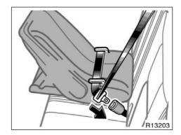
Run the lap and shoulder belt through or around the infant seat following the instructions provided by its manufacturer and insert the tab into the buckle taking care not to twist the belt. Keep the lap portion of the belt tight.
