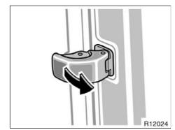
To open the rear side window, pull the latch handle toward you and swing it fully out.
