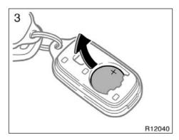
3. Remove the discharged transmitter batterv.
