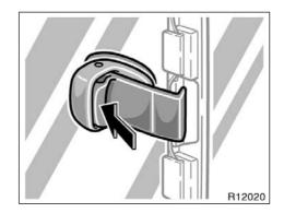
To open the rear window, push the lever and slide the window.
