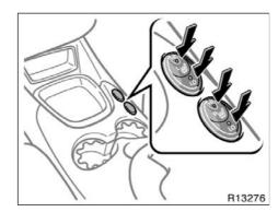
To turn on the seat heater, push the switch to "HI" (high heating temperature) or "LO" (low heating temperature).
