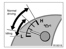
The oil pressure gauge indicates engine oil pressure when the ignition switch is on. Check it while driving to make sure that the needle is in the proper range.
