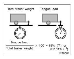
• The trailer cargo load should be distributed so that the tongue load is 15% for weight distributing hitch (\*1) or 9 to 11% for weight carrying hitch (\*2) of the total trailer weight, not exceeding the maximum load of the following. Weight distributing hitch
