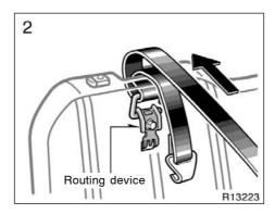
2. Route the top strap through the routing device as shown in the illustration.
