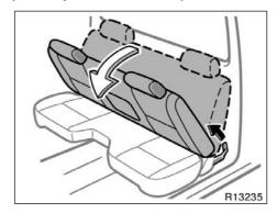
Pull the seatback lock release lever and fold down the seatback.
