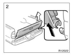
Tilt the tailgate to about 30° from vertical and pull up the right side of the tailgate to unhook the right side.
