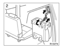
Take the holding strap out of its hole, and hook the strap onto the assist grip. Then, pull the strap on the free end to secure the seat.
