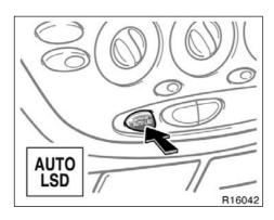
To activate the system, push the "AUTO LSD" switch under the following condition. At this time, the "AUTO LSD" indicator light will come on.
