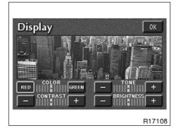
Each time you push the "+" or "-" switch, you can adjust the color, contrast, tone and brightness of the screen.
