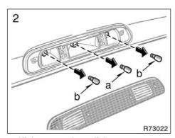
a: High mounted stoplight b: Cargo lamps
