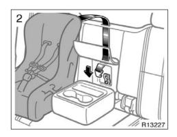
Route the top strap through the slot on top of the seat, pass the strap through the seat, then latch the hook onto the anchor bracket.
