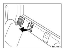
Lightly push down on the top surface of the anchor bracket cover, then pull it forward to remove.
