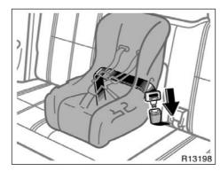
Run the center lap belt through or around the convertible seat following the instructions provided by its manufacturer and insert the tab into the buckle taking care not to twist the lap belt.
