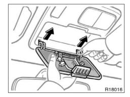
Standard and access cab models only— The auxiliary box (stored in the glove box) and garage door opener box are interchangeable.
