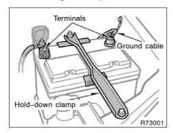
Check the battery for corroded or loose terminal connections, cracks, or loose hold-down clamp.
