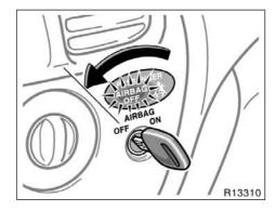
When you install a rear-facing child restraint system which belongs to a passenger risk group on the right front seat, turn the passenger airbag manual on-off switch counterclockwise to the "OFF" position. (For details, see "SRS driver airbag and front passenger airbag" in this Section.)
