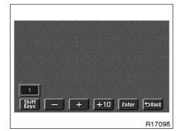
Enter the disc menu number by using the "-", "+" and "+10" switches and push the "Enter" switch. The player starts playing the disc from the entered disc menu number. The entered disc menu number will appear on the screen.
