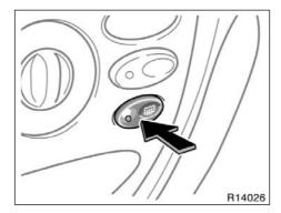
To defog or defrost the rear window, push the switch with the rear window closed.
