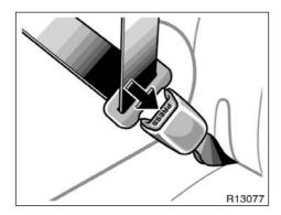
4. To remove the infant seat, press the buckle release button and allow the belt to retract completely. The belt will move freely again and be ready to work for an adult or older child passenger.
