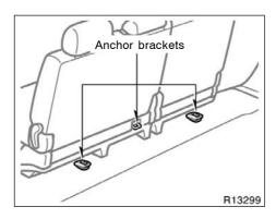
Use one anchorage on the back of rear seats and two anchorages on the floor as shown above to attach the top strap.
