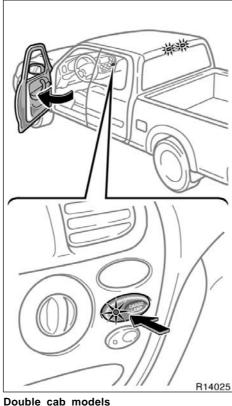
The cargo lamp is designed to light up the rear deck of your vehicle.
