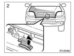
In front of the vehicle, pull up the auxiliary catch lever and lift the hood.
