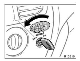
When you install a rear-facing child restraint system on the front seat, turn the passenger airbag manual on-off switch counterclockwise to the "OFF" position. (For details, see "SRS driver airbag and front passenger airbag" in this Section.)
