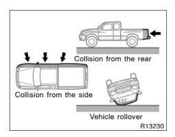
The SRS airbags are generally not designed to inflate if the vehicle is involved in a side or rear collision, if it rolls over, or if it is involved in a low-speed frontal collision. But, whenever a collision of any type causes sufficient forward deceleration of the vehicle, deployment of the SRS airbags may occur.
