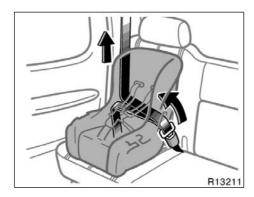
While pressing the convertible seat firmly against the seat cushion and seatback, let the shoulder belt retract as far as it will go to hold the convertible seat securely.
