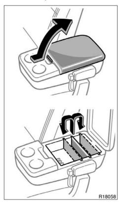
The auxiliary box is equipped with a cassette tape holder.
