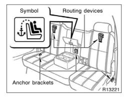
Use the routing device on the rear of the seat back and the anchor bracket on the side floor to attach the top strap.
