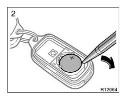
2. Remove the discharged transmitter battery.
