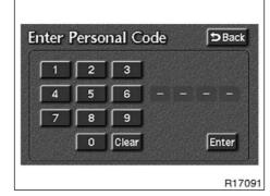
Push the number for the password and the "Enter" switch. The "Select Restriction Level" screen will appear.
