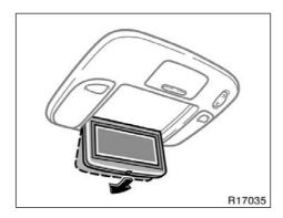
Push down the display to the desired angle.
