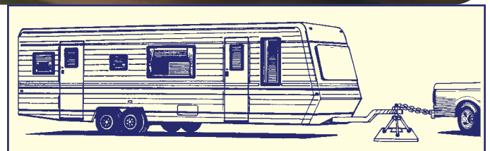
Measuring tongue weight with bathroom scale
