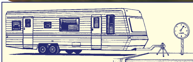
Measuring tongue weight with commercial scale
