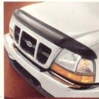
Wraparound Aero Hood/Bug Deflector is constructed of virtually unbreakable G.E. Lexan.®
