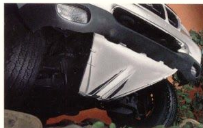
The optional XLT 4x4 Off-Road Group includes a stainless steel front suspension skid plate for added protection from rough terrain.
