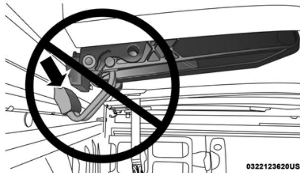
Improper Clamp Position
