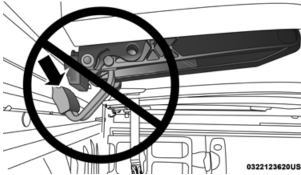
Improper Clamp Position
