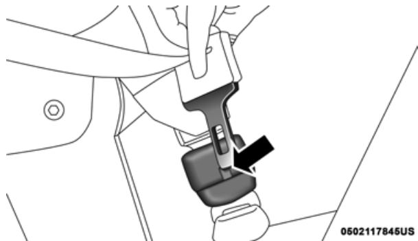
Detaching Mini-Buckle With Seat Belt Tongue
