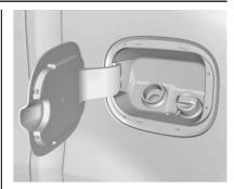
To open the fuel door, push and release the rearward center edge of the door. The capless refueling system does not have a fuel cap. Fully insert and latch the fill nozzle, then begin fueling.
