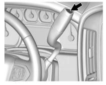
Vehicles with an automatic transmission have a Tow/Haul Mode. The Tow/Haul Mode adjusts the transmission shift pattern to reduce shift cycling. This provides increased performance, vehicle control, and enhanced transmission and engine cooling when driving
