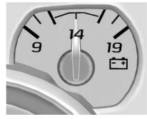
When the ignition is on, this gauge indicates the battery voltage.
