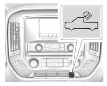
The cargo lamp provides more light in the cargo area or on the sides of the vehicle, if needed. The lights inside the pickup box and/or on the outside rearview mirrors also turn on, if equipped.
