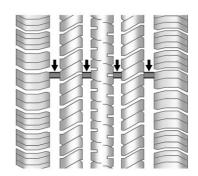
Treadwear indicators are one way to tell when it is time for new tires. Treadwear indicators appear when the tires have only 1.6 mm (1/16 in) or less of tread remaining. Some commercial truck tires may not have
