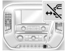
The power assist steps can be extended and extended to the tire by pressing . When extending the steps with , the kick switch is disabled.
