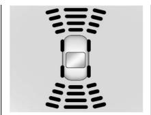
The instrument cluster may have a parking assist display with bars that show "distance to object" and object location information for the Parking Assist system. As the object gets closer, more bars light up and the bars change color from yellow to amber to red.
