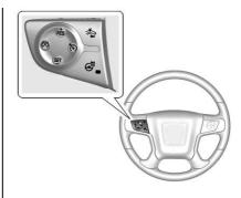
(On/Off): Press to turn the system on or off. A white indicator comes on in the instrument cluster when cruise control is on and turns off when cruise control is off.
