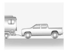
Only dinghy tow four-wheel-drive vehicles with a two-speed transfer case that have an N (Neutral) and a Four-Wheel Drive Low (4 (\dagger)) setting.
