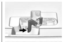
Go to the front of the vehicle to find the secondary hood release. The handle is under the front edge of the hood near the center. Push the handle to the right and at the same time raise the hood.
