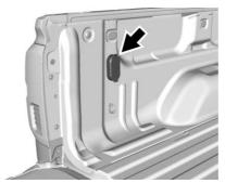
For vehicles with the 5th wheel/ gooseneck trailer package, the harness connector is mounted on the inside of the pickup bed behind the rear wheel.
