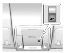
If equipped, the power sliding rear window works when the ignition has been turned to ACC/ACCESSORY or ON/RUN, or when Retained Accessory Power (RAP) is active. See Retained Accessory Power (RAP) ⇒ 281.
