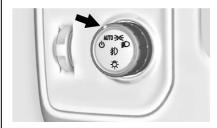
The exterior lamp control is on the instrument panel to the left of the steering wheel.
