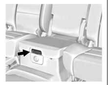
If equipped with front seat floor console storage, unlock with the ignition key, press the button, and lift to open.
