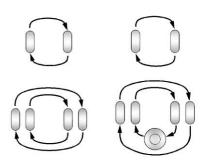
Use this rotation pattern when rotating the tires if the vehicle has polished forged aluminum dual rear wheels. The spare wheel can be used in any position in the event of a flat tire, and can be rotated with the rear inner wheels. After the flat tire is repaired, if the spare is not on one of the inner rear positions, it must be replaced by the correct wheel in the front or rear outer positions.
