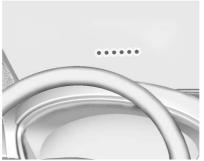
When your vehicle approaches another detected vehicle too rapidly, the red FCA display will flash on the windshield. Also, eight rapid high-pitched beeps will sound from the front, or both sides of the Safety Alert Seat will pulse five times. When this Collision Alert occurs, the brake system may prepare for driver
