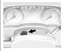
(Hazard Warning Flashers): Press this button to make the front and rear turn signal lamps flash on and off. Press again to turn the flashers off.
