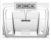
There are dome lamps in the overhead console and the headliner, if equipped.
