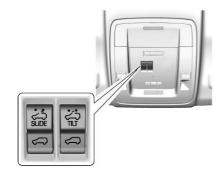
If equipped, the sunroof only operates when the ignition is in ACC/ACCESSORY or ON/RUN, or when Retained Accessory Power (RAP) is active. See Retained Accessory Power (RAP)
