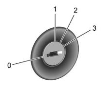
Vehicles with Key Access have an ignition switch with four different positions.
