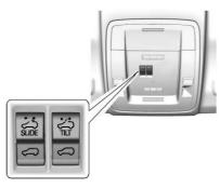
If equipped, the sunroof operates when the ignition is in ACC/ ACCESSORY or ON/RUN, or when Retained Accessory Power (RAP) is active. See Retained Accessory Power (RAP) ⇒ 281.
