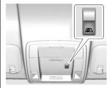
If equipped, the power sliding rear window works when the ignition has been turned to ACC/ACCESSORY or ON/RUN, or when Retained Accessory Power (RAP) is active. See Retained Accessory Power (RAP) \$ 281.
