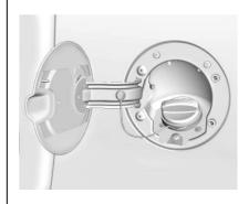
The fuel cap is behind a hinged fuel door on the driver side of the vehicle. Vehicles that have a FlexFuel badge and a yellow fuel cap can use either unleaded gasoline or ethanol fuel containing up to 85% ethanol (E85). See *E85* or FlexFuel ⇒ 319.
