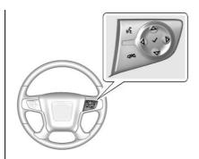
$\triangle$  or  $\nabla$ : Press to move up or down in a list. In the main view, you can press up and down to move between different info app pages.
