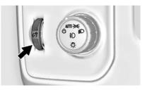
This feature controls the brightness of the steering wheel and instrument panel lights. The instrument panel illumination control is next to the exterior lamp control.
