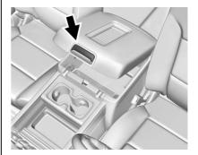
Press the latch and lift to open. Depending on the options there may be a tote compartment, accessory power outlet, auxiliary jack, and USB port(s) inside. There are openings for power cords on the edge of the storage area.
