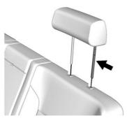
Insert the headrest posts into the holes in the top of the seatback with the longer chrome plated post toward the driver side of the vehicle. Push the headrest all the way down until it contacts the top of the seatback.
