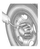
If the vehicle has wheel nut caps, loosen them by turning the wheel wrench counterclockwise. If the vehicle has a center cap with wheel nut caps, the wheel nut caps are designed to stay with the center cap after they are loosened. Remove the entire center cap.
