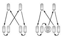
Use this rotation pattern when rotating the tires if the vehicle has dual rear wheels (except polished forged aluminum wheels).
