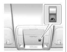
If equipped, the power sliding rear window works when the ignition has been turned to ACC/ACCESSORY or ON/RUN, or when Retained Accessory Power (RAP) is active. See Retained Accessory Power (RAP) on page 9-28.
