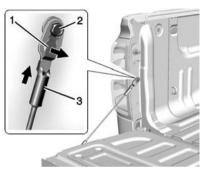
Raise the tailgate and support it firmly. Pull out and hold the cable retaining clip (1). Push the cable (3) up and off of the bolt (2). Repeat on the other side.
