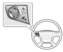
The FCA control is on the steering wheel. Press to set the FCA timing to Far, Medium, Near, or Off. The first button press shows the current setting on the DIC. Additional button presses will change this setting. The chosen setting will remain until it is changed and will affect the timing of both the Collision Alert and the Tailgating Alert features. The timing of both alerts will vary based on vehicle speed. The faster the vehicle speed, the farther away the alert will occur.
