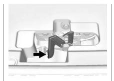
Go to the front of the vehicle to find the secondary hood release. The handle is under the front edge of the hood near the center. Push the handle to the right and at the same time raise the hood. Before closing the hood, be sure all the filler caps are on properly. Then bring the hood from full open to within 15 cm (6 in) from the closed position, pause, and push the front center of the hood with a swift, firm motion to fully close the hood.
