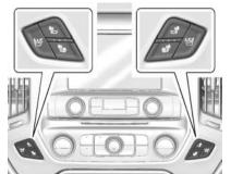
Heated and Cooled Seat Buttons Shown, Heated Seat Buttons Similar
