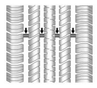
Treadwear indicators are one way to tell when it is time for new tires. Treadwear indicators appear when the tires have only 1.6 mm (1/16 in) or less of tread remaining. Some commercial truck tires may not have treadwear indicators. See *Tire Inspection on page 10-67* and *Tire Rotation on page 10-67* for additional information.
