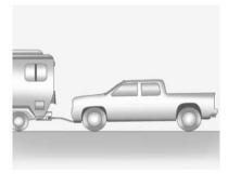
Only dinghy tow four-wheel-drive vehicles with a two-speed transfer case that have an N (Neutral) and a Four-Wheel Drive Low (4 (\$\dpsi\$) setting.
