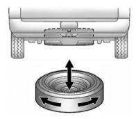
Make sure the tire is stored securely. Push, pull, and then try to turn the tire. If the tire moves, use the wheel wrench to tighten the cable. 8. Reinstall the spare tire lock, if the vehicle has one.
