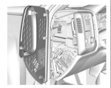
The left instrument panel fuse block access door is on the driver side edge of the instrument panel.
