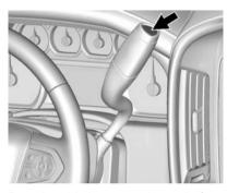
Pressing this button at the end of the shift lever turns on and off the Tow/Haul Mode.
