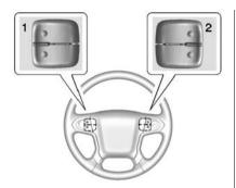
The favorite and volume switches are on the back of the steering wheel.
