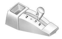
Move the lever to shift into and out of four-wheel drive.
