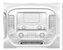
The switch used to adjust the pedals is on the center stack, below the climate controls.
