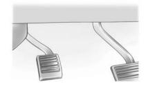
For vehicles without a release handle, set the parking brake by holding the regular brake pedal down, then pushing down the parking brake pedal.
