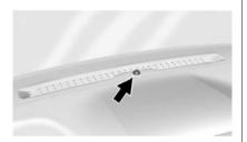
The solar sensor, located in the defrost grille in the middle of the instrument panel, monitors the solar heat. Do not cover the solar sensor or the system will not work properly.
