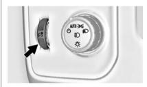
This feature controls the brightness of the steering wheel and instrument panel lights. The instrument panel illumination control is next to the exterior lamp control.
