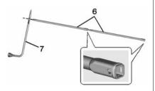
Assemble the wheel wrench (7) and the two jack handle extensions (6), as shown.
