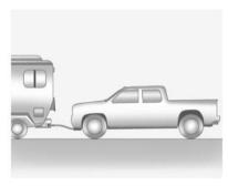
Only dinghy tow four-wheel-drive vehicles with a two-speed transfer case that have an N (Neutral) and a Four-Wheel Drive Low (4 (1) setting.
