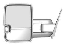
If equipped, adjust trailer-tow mirrors for a clear view of the area behind you. Manually pull out the mirror head to extend it for better visibility when towing a trailer.
