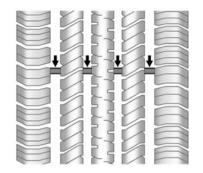
Treadwear indicators are one way to tell when it is time for new tires. Treadwear indicators appear when the tires have only 1.6 mm (1/16 in) or less of tread remaining. Some commercial truck tires may not have treadwear indicators. See *Tire Inspection on page 10-69* and *Tire Rotation on page 10-69* for additional information.
