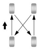
Use this rotation pattern when rotating the tires if the vehicle has single rear wheels.
