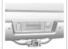
For vehicles equipped with heavy-duty trailering, the harness connector is mounted in the bumper. The seven-wire harness contains the following trailer circuits:
