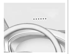
When your vehicle approaches another detected vehicle too rapidly, the red FCA display will flash on the windshield. Also, eight rapid high-pitched beeps will sound from the front, or both sides of the Safety Alert Seat will pulse five times.
