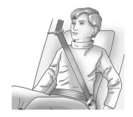
4. Buckle, position, and release the safety belt as described previously in this section. Make sure the shoulder portion of the belt is on the shoulder and not falling off of it. The belt should be close to, but not contacting, the neck
