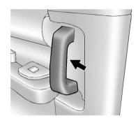
To open a rear access door from the inside, first open the front door. Then, use the handle located on the inside of the rear access door to open.
