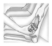
For crew cab second row seatings positions, tilt the latch plate to adjust the belt if needed.
