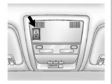
On vehicles with a sunroof, the sunroof only operates when the ignition is in the ACC/ACCESSORY or ON/RUN or the Retained Accessory Power (RAP) is active. See Retained Accessory Power (RAP) on page 9-32 for more information.
