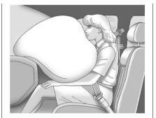
The right front passenger airbag is in the instrument panel on the passenger side.
