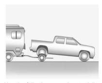
Use the following procedure to dolly tow a two-wheel-drive vehicle from the rear:
