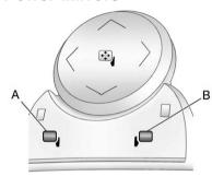
Vehicles with outside power mirrors have controls located on the driver door.
