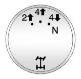
This transfer case knob is located next to the steering column.
