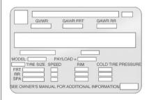
A vehicle specific Certification/ Tire label is found on the rear edge of the driver door. The label shows the size of your vehicle's original tires and the inflation pressures needed to obtain the gross weight capacity of your vehicle. This is called Gross Vehicle Weight Rating (GVWR). The GVWR includes the weight of the vehicle, all occupants, fuel, and cargo.
