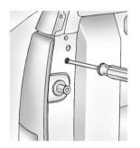
Remove the two rear lamp assembly screws near the tailgate latch strikerpost and pull rearward until disengaging the two outer pins on the taillamp assembly from the vehicle.
