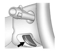
The tilt lever is located on the lower left side of the steering column.
