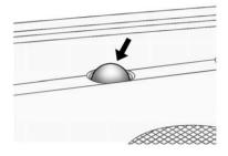
The solar sensor, located in the defrost grille in the middle of the instrument panel, monitors the solar heat. Do not cover the solar sensor or the system will not work properly.
