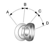
The ignition switch has four different positions.
