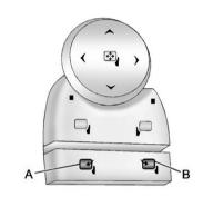
Vehicles with outside power foldaway mirrors have controls on the driver door.
