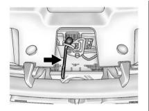
Go to the front of the vehicle and locate the secondary hood release. This is located under the hood, near the center of the grille.
