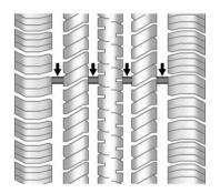
Treadwear indicators are one way to tell when it is time for new tires. Treadwear indicators appear when the tires have only 1.6 mm (1/16 in) or less of tread remaining. Some commercial truck tires may not have treadwear indicators.
