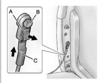
Raise the tailgate slightly, pull out and hold the cable retaining clip (A). Push the cable (C) up and off of the bolt (B). Repeat on the other side.
