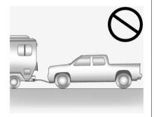
Notice: If the vehicle is towed with all four wheels on the ground, the drivetrain components could be damaged. The repairs would not be covered by the vehicle warranty. Do not tow the vehicle with all four wheels on the ground.
