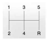
If the vehicle is equipped with a manual transmission, this is the shift pattern.
