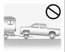
Notice: If a two-wheel drive vehicle is towed with the rear wheels on the ground, the transmission could be damaged. The repairs would not be covered by the vehicle warranty. Never tow the vehicle with the rear wheels on the ground.
