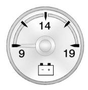
This gauge indicates the battery voltage when the ignition is turned on.
