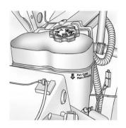
The coolant level should be at or above the FULL COLD mark. If it is not, there may be a leak in the cooling system.
