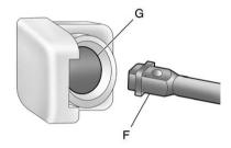
Insert the hoist end (open end) (F) of the extension through the hole (G) in the rear bumper.
