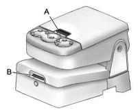
Pull the lever (A) up to access the upper storage area. Raise the upper storage bin, then pull the lever (B) up to access the lower storage area. Use the key to lock and unlock the lower storage area.
