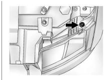
Locate the vertical headlamp aiming screws, which are under the hood near each headlamp assembly.
