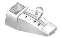
This transfer case shift lever is on the floor to the right of the driver.
