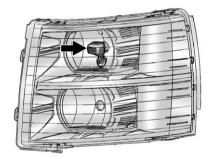
2. Locate the aim dot on the lens of the low-beam headlamp.
