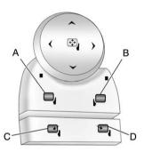
Vehicles with outside power mirrors and foldaway mirrors have controls located on the driver door.
