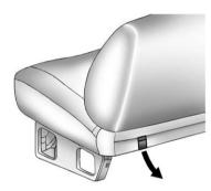
Pull one of the release levers, at each end of the seat on the lower rear of the seatback, completely out.
