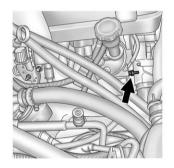
If your vehicle has a gasoline engine, the remote negative (-) terminal is a stud located on the right front of the engine, where the negative battery cable attaches.
