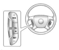
(On/Off): Press to turn the system on or off. The indicator light is on when cruise control is on and turns off when cruise control is off.
