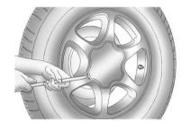
If the wheel has a smooth center cap, place the chisel end of the wheel wrench in the slot on the wheel, and gently pry it out.
