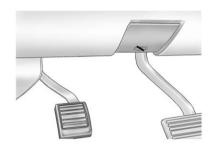
For vehicles with a release handle, set the parking brake by holding the regular brake pedal down, then pushing down the parking brake pedal.
