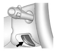
The tilt lever is located on the lower left side of the steering column.
