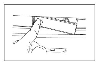
Press and hold the driver's side of the handle in and pull out on the exposed portion of the handle to access the storage area.
