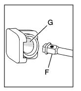
Insert the hoist end (F) through the hole (G) in the rear bumper and onto the hoist shaft.
