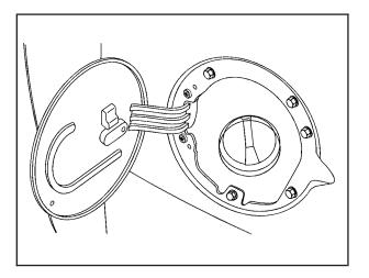
The tethered fuel cap is located behind a hinged fuel door on the driver side of the vehicle. If the vehicle has E85 fuel capability, the fuel cap will be yellow and state that E85 or gasoline can be used. See *Fuel E85* (85% Ethanol) on page 5-8.
