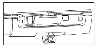
For vehicles equipped with heavy duty trailering, the harness is connected to a bracket on the hitch platform. The seven-wire harness contains the following trailer circuits:
