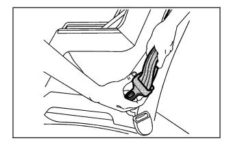
For crew cab second row seatings positions, tilt the latch plate to adjust the belt if needed.
