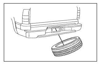
6. Tilt the tire toward the vehicle with some slack in the cable to access the tire/wheel retainer. Separate the retainer from the guide pin by sliding the retainer up the pin while pressing down on the latch.
