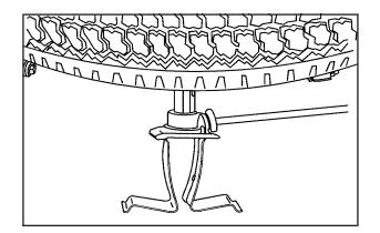
8. Attach the jack handle, extension, and wheel wrench to the jack and place it (with the wheel blocks) under the vehicle toward the front of the rear bumper.
