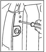
near the tailgate latch strikerpost and pull out the lamp assembly.
