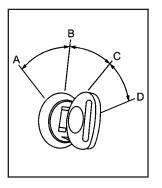
The ignition switch has four different positions.
