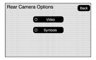
4. Select the Video screen button. When the Video screen button is highlighted the RVC system is on.
