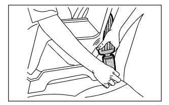
Push the latch plate into the buckle until it clicks. Position the release button so that the safety belt could be quickly unbuckled if necessary.
