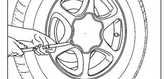
If the vehicle has a center cap with wheel nut caps, the wheel nut caps are designed to stay with the center cap after they are loosened. Remove the entire center cap.
