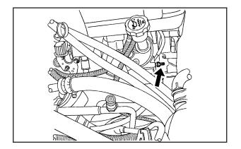
The remote negative (-) terminal is a stud located on the right front passenger side of the engine, where the negative battery cable attaches. See *Engine Compartment Overview on page 5-14*.
