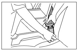
Push the latch plate into the buckle until it clicks. Position the release button so that the safety belt could be quickly unbuckled if necessary.
