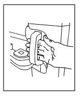
To open a rear access door from the inside, the front door must be opened first. Then, use the handle located on the inside of the rear access door to open.
