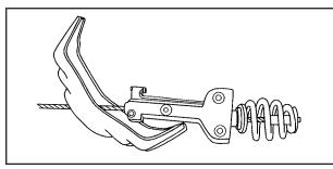
2. Separate the tire/wheel retainer (D) from the guide pin. Pull the pin through the center of the wheel. Tilt the retainer down and through the center wheel opening.
