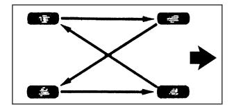
If your vehicle has single rear wheels and the tread design for the front tires is the same as the rear tires, use the rotation pattern shown here when rotating the tires.
