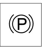
A parking brake symbol is located next to the N (Neutral) symbol as a reminder to set the parking brake before shifting the transfer case into N (Neutral).
