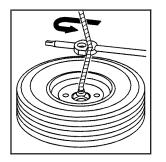
Use the wheel wrench hook which allows you to pull the hoist cable towards you to assist in reaching the spare tire.
