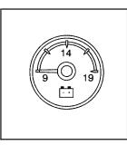
For vehicles with a voltmeter gage, this gage indicates the battery voltage when the ignition is turned on.
