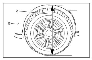
When using a weight-distributing hitch, the hitch must be adjusted so the distance (A) remains the same both before and after coupling the trailer to the tow vehicle.
