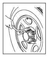
If your vehicle has wheel nut caps, loosen them by turning the wheel wrench counterclockwise.
