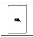
On vehicles with a power sliding rear window, the switch is located in the overhead console.
