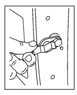
Raise the tailgate slightly and release both retaining cable clips. To release the retaining cable clips, lift the cable so it points straight out. Lift the clip over the bolt, and push the cable forward then rotate down. 2. With the tailgate about halfway open, lift the right edge of the tailgate from the lower pivot.
