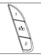
The controls for this feature are located on the driver's door panel, and are used to program and recall memory settings for the driver's seat, outside mirrors, and the adjustable throttle and brake pedal. To save seating positions in memory:
