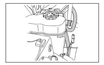
The coolant level should be at or above the FULL COLD mark. If it is not, you may have a leak in the cooling system.
