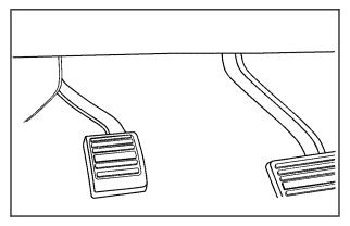
For vehicles without a release handle, set the parking brake by holding the regular brake pedal down, then pushing down the parking brake pedal. If the ignition is on, the brake system warning light will come on. See *Brake System Warning Light on page 3-42*.
