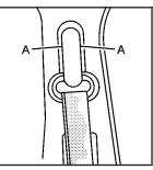
To move the adjuster down for the regular and crew cabs, squeeze the buttons (A) on the sides of the height adjuster and move the height adjuster to the desired position.
