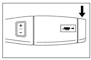
Vehicles with an Allison or Hydra-Matic<sup>®</sup> 6-speed automatic transmission<sup>®</sup> have a tow/haul mode. The tow/haul mode adjusts the transmission shift pattern to reduce shift cycling, providing increased performance, vehicle control, and transmission cooling when towing or hauling heavy loads.
