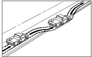
If the level of the shoulder is only slightly below the pavement, recovery should be fairly easy. Ease off the accelerator and then, if there is nothing in the way, steer so that the vehicle straddles the edge of the pavement. Turn the steering wheel 3 to 5 inches, 8 to 13 cm, (about one-eighth turn) until the right front tire contacts the pavement edge. Then turn the steering wheel to go straight down the roadway.
