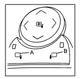
Vehicles with outside power mirrors have controls located on the driver door armrest.
