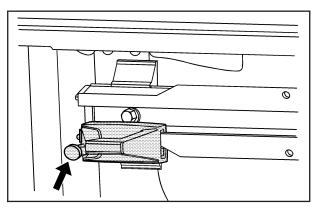
To adjust a tie-down, pull the locator pin out and move the tie-down to another location making sure the locator pin lines up with a locator hole on the rail. The tie-down pin may not be installed correctly if the pin does not line up, turn it over and reinstall. The tie-down will not move when the pin is installed completely. The maximum load for each rail is 500 lbs (227 kg).
