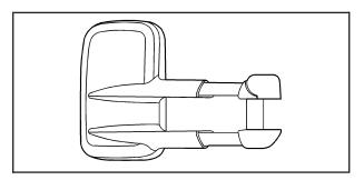
If your vehicle has trailer towing type mirrors, they can be adjusted so you can have a clear view of the objects behind you. Manually pull out the mirror head to extend it for better visibility when towing a trailer.
