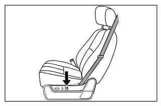
If the seats have power lumbar, the controls used to operate this feature are located on the outboard side of the seats.
