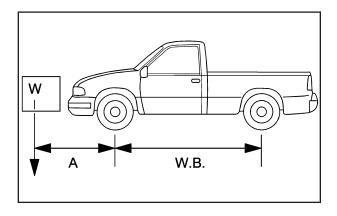
$(W \times (A + W.B.)) /W.B.=$  Weight the accessory is adding to the front axle.
