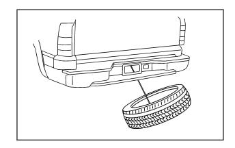
Tilt the tire toward the vehicle with some slack in the cable to access the tire/wheel retainer.
