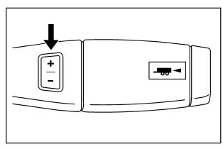
Your vehicle may have a Range Selection Mode. The Range Selection Mode helps control the vehicle's transmission and vehicle speed while driving down hill or towing a trailer by letting you select a desired range of gears.
