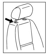
Pull the head restraint up to raise it. To lower the head restraint, press the release button, located on the top of the seatback, while you push the head restraint down.
