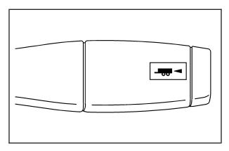
If your vehicle has an automatic transmission, it has a tow/haul mode. If your vehicle has an Allison or Hydra-Matic® 6-speed automatic transmission see "Tow/Haul Mode (Allison or Hydra-Matic® 6-Speed Automatic Transmission®) following. The tow/haul mode adjusts the transmission shift pattern to reduce shift cycling, providing increased performance, vehicle control, and transmission cooling when towing or hauling heavy loads.
