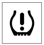
When a low tire pressure condition is detected, the TPMS will illuminate the low tire pressure warning symbol located on the instrument panel cluster.
