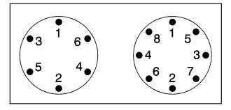
12. Tighten the nuts firmly in a crisscross sequence as shown by turning the wheel wrench clockwise.
