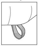
Pull up on the front of the seat cushion while pulling down on the release strap, located under the seat cushion.
