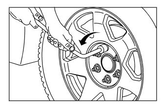
Use the wheel wrench and turn it counterclockwise to loosen the wheel nuts. Do not remove the wheel nuts yet.
