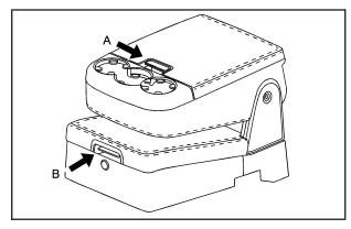
To access the upper storage area, pull lever (A) up. To access the lower storage area, raise the upper storage bin, then pull lever (B) up. Use the key to lock and unlock the lower storage area.
