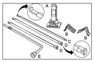
The tools you will be using include the jack (A), the wheel blocks (B), the jack handle (C), the jack handle extensions (D), and the wheel wrench (E).
