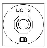
The brake master cylinder reservoir is filled with DOT-3 brake fluid. See Engine Compartment Overview on page 5-16 for the location of the reservoir.
