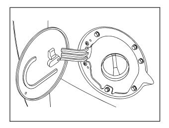
The tethered fuel cap is located behind a hinged fuel door on the driver's side of the vehicle. If the vehicle has E85 fuel capability, a yellow cap with the words "E85 / Gasoline" can be seen.
