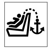
For regular cab models, there is an anchor symbol on the covers to assist you in locating the top tether anchors.
