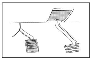
To release the parking brake, hold the regular brake pedal down. Then pull the bottom edge of the lever, with the parking brake symbol and located above the parking brake pedal.
