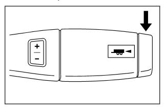
If your vehicle has an Allison or Hydra-Matic® 6-speed automatic transmission®, it has a tow/haul mode. The tow/haul mode adjusts the transmission shift pattern to reduce shift cycling, providing increased performance, vehicle control, and transmission cooling when towing or hauling heavy loads.
