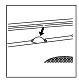
The solar sensor, located in the defrost grille, in the middle of the instrument panel, monitors the solar radiation. Do not cover the solar sensor or the system will not work properly.
