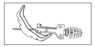
Once the retainer is separated from the guide pin, tilt the retainer and pull it through the center of the wheel along with the cable and guide latch.
