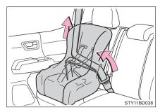
5 If the child restraint has a top tether strap, the top tether strap should be latched onto the top tether strap anchor. (→P. 66, 68)
