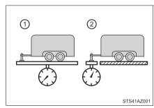
If using a weight distributing hitch when towing, return the front axle to the same weight as before the trailer connection.
