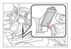
3 Remove the fuse with the pullout tool.
