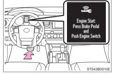
Press the engine switch shortly and firmly.
