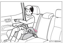
Check that the shoulder belt is correctly positioned over the child's shoulder and that the lap belt is as low as possible.  $(\rightarrow P. 30)$
