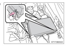
Under the instrument panel Remove the cover.
