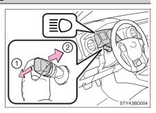
You can flash the high beams with the headlights on or off.
