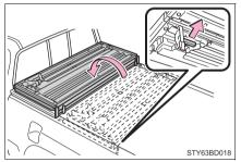
4 Secure by using the storage straps.
