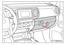
Remove the cover by sliding up and then pull the cover toward you.
