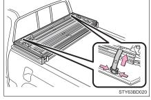
2 Close the tonneau cover and push down on the top surface (latch position) until it clicks.
