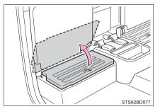
4 Unhook the rubber band and remove the tool bag.
