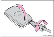
Remove the depleted battery.
