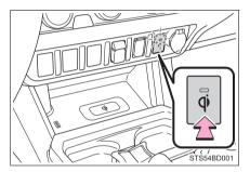
2 Place a mobile device on the tray as shown in the illustration.
