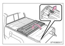
3 Pull the lever and lift to open the center tonneau cover.
