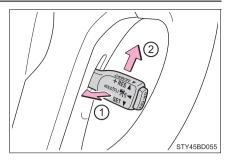
(2) Pushing the lever up resumes the cruise control and returns vehicle speed to the set speed.
