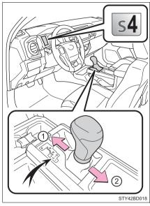
The initial shift range in S mode is set automatically to 5 or 4 according to vehicle speed. However, the initial shift range may be set to 3 if the AI-SHIFT has operated while the shift lever was in the D position.  $(\rightarrow P. 212)$
