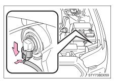
2 Turn the bulb base counter-clockwise.
