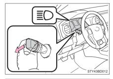
2 Press the Automatic High Beam switch.
