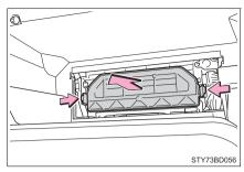
5 Pull the filter out of the filter outlet.
