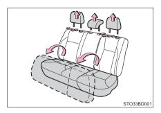
Attach the head restraints to the holders located on the back sides of the bottom cushions.
