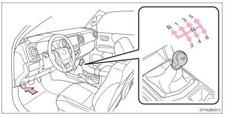
Fully depress the clutch pedal before operating the shift lever, and then release it slowly.
