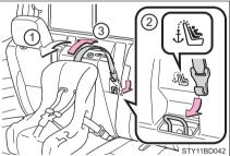
3 Secure the child restraint system using the seat belt or the lower anchors, ant tighten the top tether strap.
