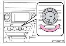
The air conditioning will automatically turn on and the air intake selector will be set to recirculated air mode.
