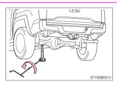
4 Firmly tighten each nut two or three times in the order shown in the illustration.
