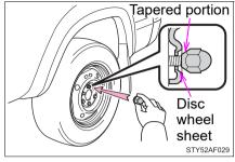
▶ Replacing an aluminum wheel with a spare steel wheel
