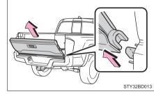
3 Slide the tailgate a little to the right to unhook the left side being mindful of tailgate right-hand side clearance to vehicle's rear bumper.
