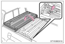
4 Secure by using the storage straps.
