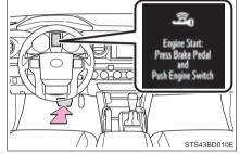
Press the engine switch shortly and firmly.
