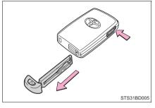
After using the mechanical key, store it in the electronic key. Carry the mechanical key together with the electronic key. If the electronic key battery is depleted or the entry function does not operate properly, you will need the mechanical key.  $(\rightarrow P. 611)$
