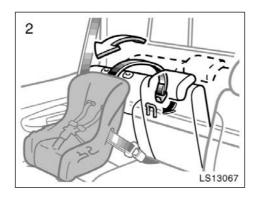
2. Pull the seatback release strap and swing the seatback forward slightly, then latch the hook onto the anchor bracket.
