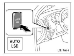
To activate the system, push the "AUTO LSD" switch with the vehicle stopped.
