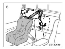
Pull the seatback release lever and swing the seatback forward slightly.
