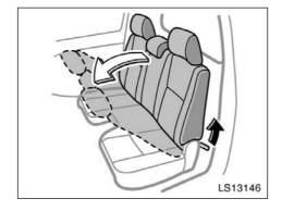
Pull the seatback lock release lever and fold down the seatback.
