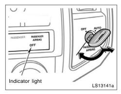
This off switch is designed to disable the front passenger airbag in order to allow usage, if necessary, of a member of a passenger risk group identified in TABLE 1 is occupying the right front passenger seating position (bench seat) or front passenger seating position (separate seats). (For details, see "SRS driver airbag and front passenger airbag" on page 55 in this Section.)
