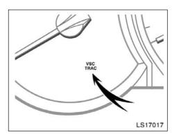
If there is any abnormality in the system, the "VSC TRAC" warning light will come on. When the "DAC" switch is pushed, the downhill assist control system indicator light also flash.
