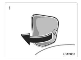
To open the fuel filler door, pull the door toward out as shown.
