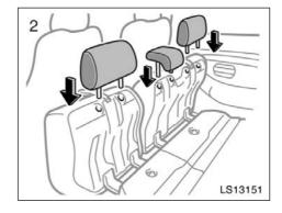
2. Attach the head restraints to the holders located on the back sides of the bottom cushions.
