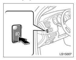
To turn on the front fog lights, push the switch. They will come on when the headlights are turned on.
