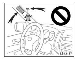
• Do not attach a microphone or any other device or object around the area where the curtain shield airbag activates such as on the windshield glass, side door glass, front and rear pillars, roof side rail and assist grips. When the curtain shield airbags inflate, the microphone or other device or object will be thrown away with great force or the curtain shield airbags may not activate correctly, resulting in death or serious injury.
