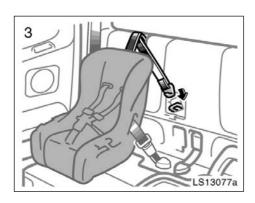
Latch the hook onto the rear lower anchor bracket and tighten the top strap.
