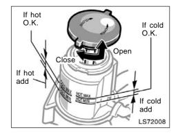
Check the fluid level through the reservoir. If necessary, add automatic transmission fluid DEXRON®II or III.
