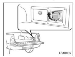
This power outlet is designed for use as a power supply for electric appliances.
