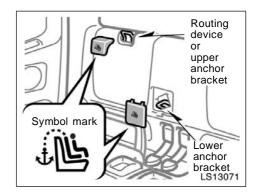
Use the routing device and the anchor bracket to attach the top strap.
