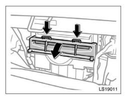
3. Push down on the tabs and open the filter door.
