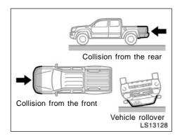
The SRS side airbags and curtain shield airbags are not generally designed to inflate if the vehicle is involved in a front or rear collision, if it rolls over, or if it is involved in a low-speed side collision.
