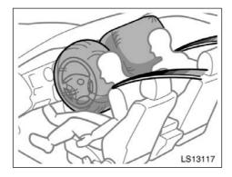
The SRS (Supplemental Restraint System) front airbags are designed to provide further protection for the driver and right front passenger (bench seat) or front passenger (separate seats) in addition to the primary safety protection provided by the seat belts.
