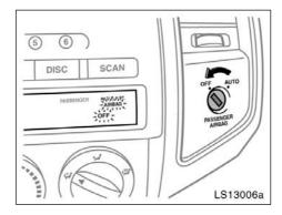
When you install a rear-facing child restraint system which belongs to a passenger risk group on the right front passenger seat (bench seat) or front passenger seat (separate seats), turn the passenger airbag off switch counterclockwise to the "OFF" position and remove the key. (For details, see "SRS driver airbag and front passenger airbag" on page 55 in this Section.)
