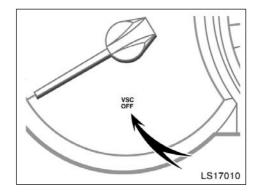
The vehicle stability control system automatically turns off, and the "VSC OFF" indicator light is illuminated, when either one of the following conditions applies:
