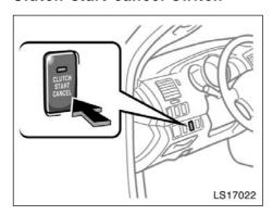
Never use the switch for normal engine starting. Be sure to follow the starting procedure instructed in "How to start the engine" on page 298 in Section 3.
