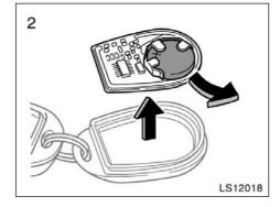
2. Remove the circuit board, then remove the discharged transmitter battery.
