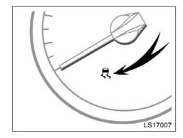
When the hill-start assist control system is operating, the slip indicator light flashes and an alarm sounds intermittently. At the same time, the stop lamps and high mounted stoplight are lit.
