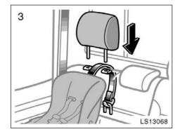
3. Fix the child restraint system with the seat belt and tighten the top strap.
