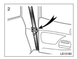
2. Make sure the shoulder belt passes through the hanger when folding the rear seat.
