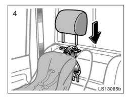
4. Fix the child restraint system with the seat belt and tighten the top strap.
