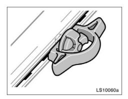
5. Check the tie-down cleat to confirm that it is locked into a detent and securely mounted to the deck rail system.
