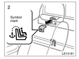
2. Lightly push down on the top surface of the routing device cover with the symbol mark shown in the illustration, then pull it forward to remove.
