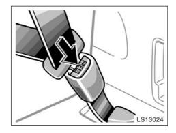
2. To remove the booster seat, press the buckle release button and allow the belt to retract.
