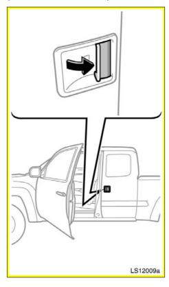
For easy access to the rear seat, open the access door (rear door).
