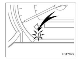
When initializing the system, make sure the low tire pressure warning light blinks three times. If the warning light does not blink three times, initialization failed and the tire pressure warning system will not function properly. In this case, initialize the system again.
