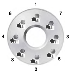
8-lug nut torque sequence
