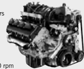
**CONFIGURATION:** 90-degree V8, liquid-cooled
