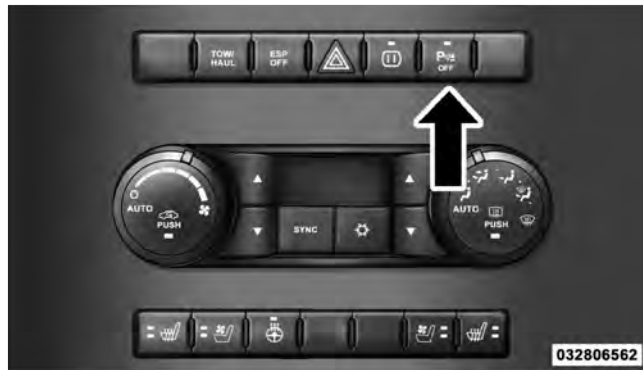
Park Assist Switch
