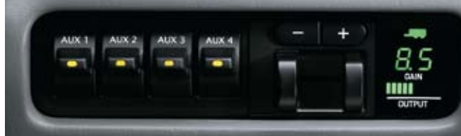
Trailer Brake Controller shown to the right of Upfitter Switches, which are standard on F-350/F-450/F-550 Chassis Cab; optional on F-250/F-350 Pickup (66S).
