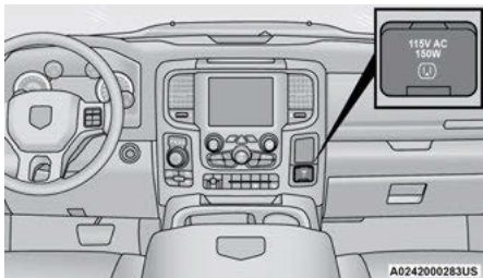
Power Inverter Outlet
