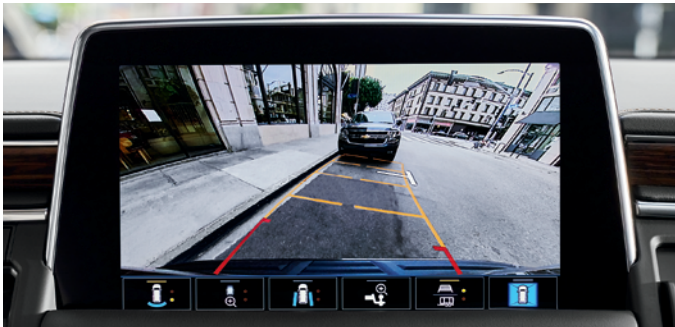
Rear Camera View Displays a rear view to assist with parking and tight maneuvers.
