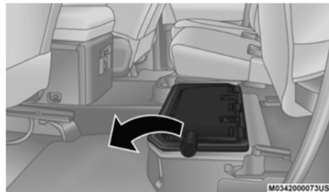
**Unfolding The Load Floor**
