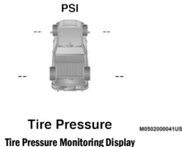
If the ignition switch is cycled, this sequence will repeat, providing the system fault still exists. If the system fault no longer exists, the "TPMS Warning Light" will no longer flash, and the "SERVICE TPM SYSTEM" message will no longer display, and a pressure value will display in place of the dashes.
