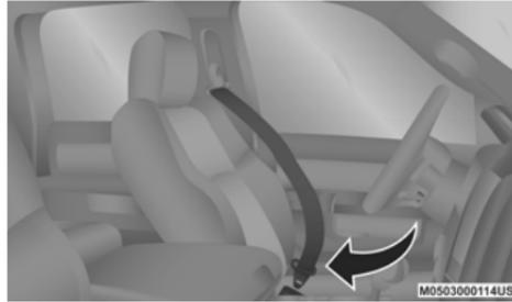
**Inserting Latch Plate Into Buckle**
