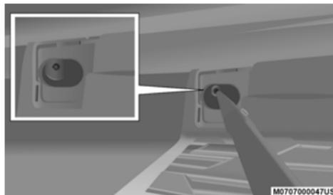
**Winch Mechanism Tube**
