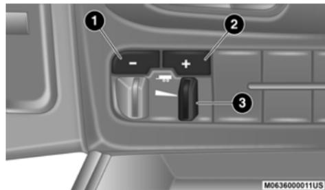
Integrated Trailer Brake Module (ITBM)
