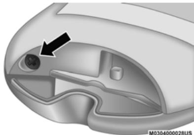
Remove Screw (If Equipped) From Key Fob Case
