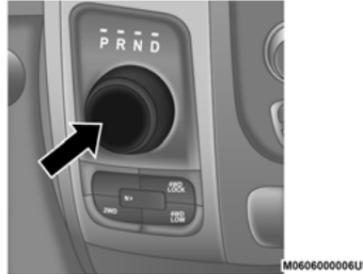
**Electronic Transmission Gear Selector**
