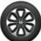
20-inch Cast-Aluminum Premium Paint/Partial Clad Standard on Limited (WRH)
