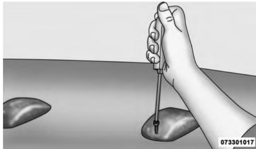
Removing Rear Screw From Clearance Lamp
