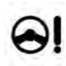
This telltale is on when the Electric Power Steering is not operating and needs service.
