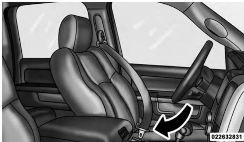
Inserting Latch Plate Into Buckle
