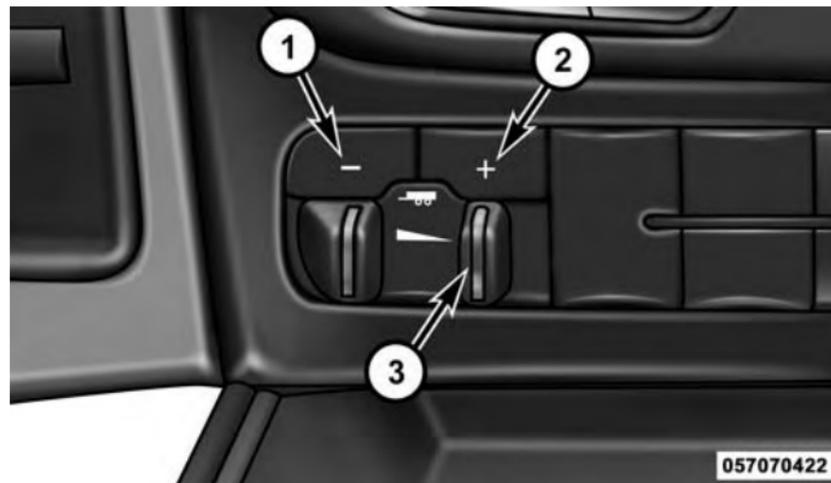
Integrated Trailer Brake Module (ITBM)
