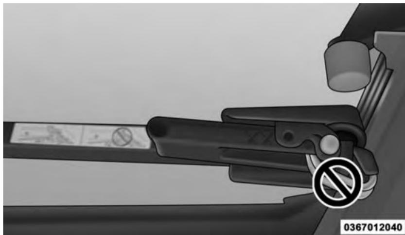
Improper Clamp Wire Released Position
