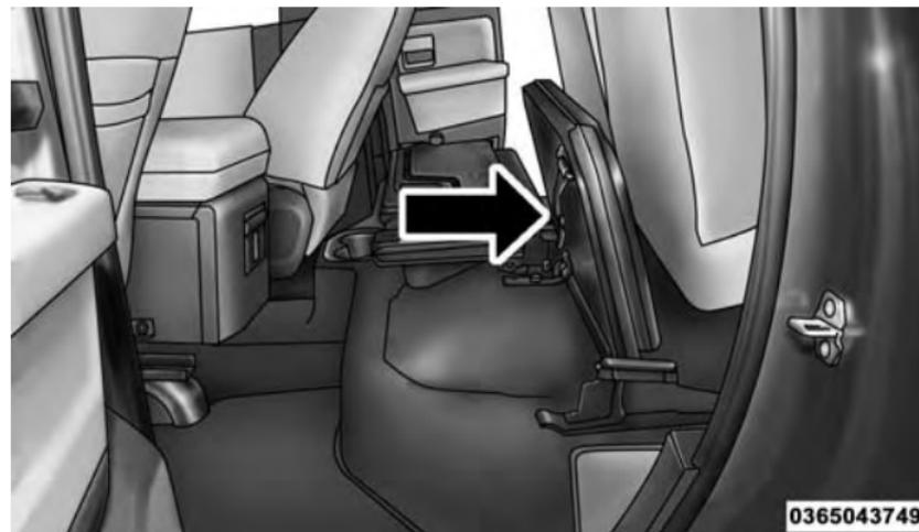
Load Floor Securing Straps/Crew Cab®
