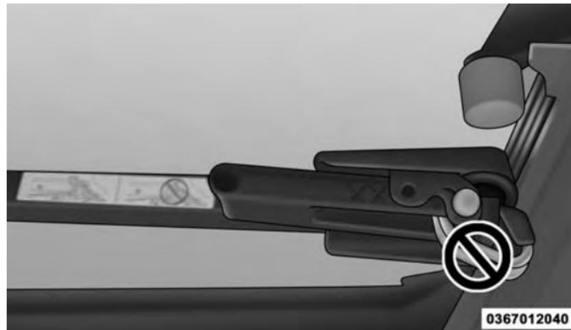
Improper Clamp Position
