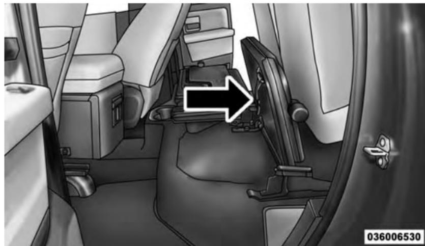
Load Floor Securing Straps/Quad Cab®
