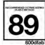
This engine is designed to meet all emissions regulations and provide satisfactory fuel economy and performance when using high quality unleaded gasoline having an octane range of 87 to 89. The manufacturer recommends the use of 89 octane for optimum performance. The use of premium gasoline (Over 89 octane) is not recommended, as it will not provide any benefit over regular gasoline in these engines.
