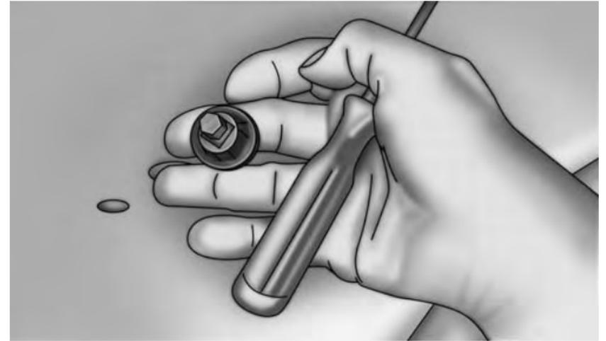
Removing The Bulb From The Bulb Socket
