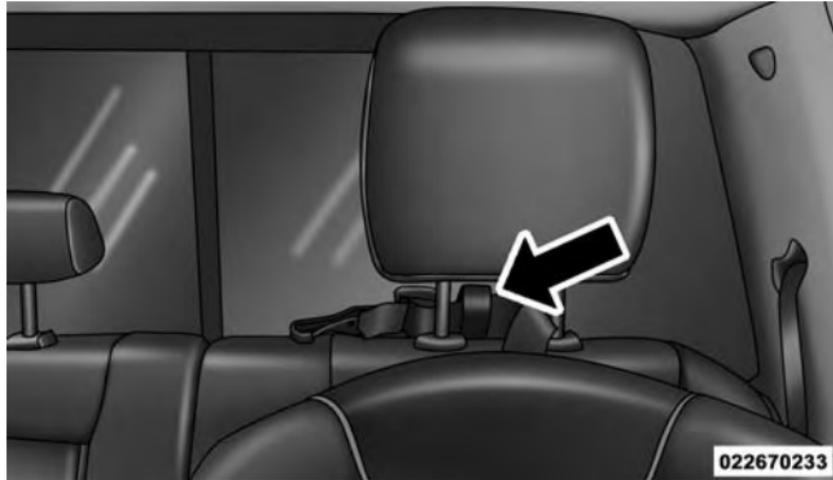
Tether Strap Through Outboard Tether Strap Loop
