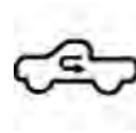
When outside air contains smoke, odors, or high humidity, or if rapid cooling is desired, you may wish to recirculate interior air by pressing the RECIRCULATION control button on the touchscreen or faceplate. Recirculation mode should only be used temporarily. The recirculation LED button on the faceplate will illuminate when either button is selected. Push either button a second time to turn off the Recirculation mode LED and allow outside air into the vehicle.
