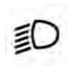
To turn on the headlights, rotate the headlight switch clockwise to the headlight position. When the headlight switch is on, the parking lights, taillights, license plate light and instrument panel lights are also turned on. To turn off the headlights, rotate the headlight switch back to the O (Off) position.
