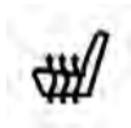
Push the switch once to select HI-level heating. Push the switch a second time to select LO-level heating. Push the switch a third time to shut the heating elements OFF.
