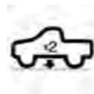
For easy entry and loading, your vehicle can be lowered by pushing the Key Fob air suspension lowering button two times. When Remote key FOB lowering is requested, the vehicle will
