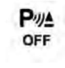
When the ParkSense switch is pushed to disable the system, the instrument cluster will display the “PARKSENSE OFF” message for approximately five seconds. Refer to “Electronic Vehicle Information Center (EVIC) or Driver Information Display (DID)” in “Understanding Your Instrument Panel” for further information. When the shift lever is moved to REVERSE and the system is disabled, the EVIC/DID will display the “PARKSENSE OFF” message for as long as the vehicle is in REVERSE.
