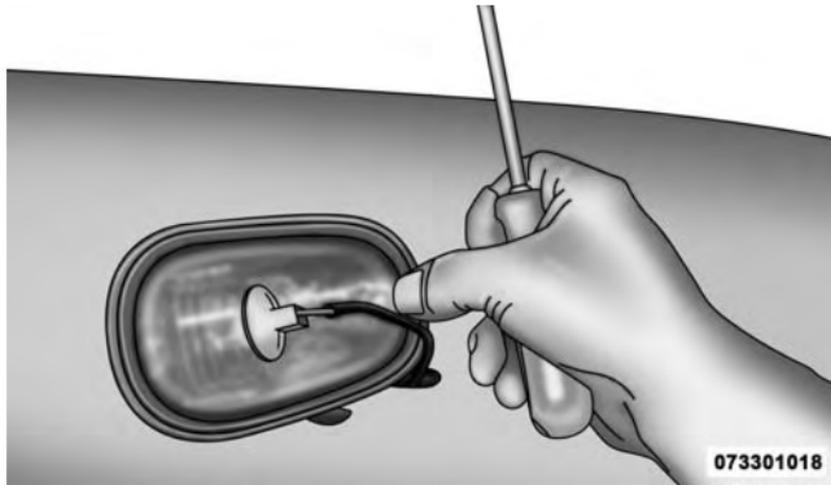
Removing Bulb Socket From Clearance Lamp
