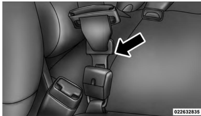
**Inserting Latch Plate**
