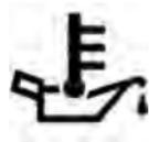
This telltale indicates engine oil temperature is high. If the light turns on while driving, stop the vehicle and shut off the engine as soon as possible.
