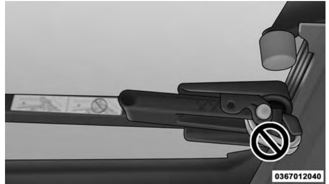
Improper Clamp Position
