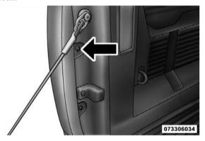
2. Pull the outboard side of the lamp rearward far enough to unsnap the two receptacles on the outboard side of the lamp housing from the two plastic snap post retainers in the outer box side panel.
