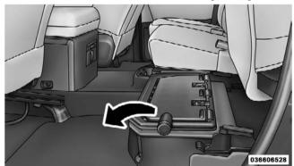
**Unfolding The Load Floor**
