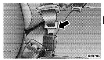
**Inserting Latch Plate**
