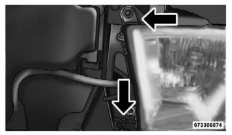
7. Reach into the front wheel house ahead of the front wheel, remove the fastener, and lift the cover over the access hole in the front of the wheel house splash shield. Access to the rear of the lamp can be gained through this access hole.
