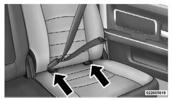
Quad Cab®/Crew Cab Rear Outboard Seats Driver Side Child restraint systems having attachments designed to connect to the lower anchorages are now available. Child restraints having tether straps and hooks for connection to the seat back tether anchorage have been available for
