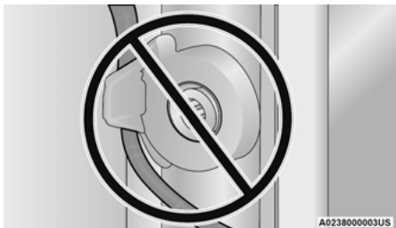
Incorrectly Seated Tailgate Strap
