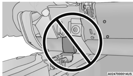
Incorrectly Seated Retainer
